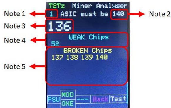
Figure 20: the test result of T2Tz hashboard with condition (Mode1)
