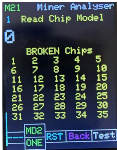
Figure 18, testing READ CHIP MODEL command for whatsmineer hashboards (MODE2)
